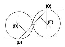
Use the Trim command to trim away any excess arc segments to form the ogee curve. This forms the frame of the ogee for the construction of objects such as the wrench illustrated at the right.
